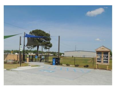
While the City of Dunn Dog Park has an ADA accessible space that is van accessible, the access aisle should be increased from a 5' width to an 8' width to be fully compliant.
