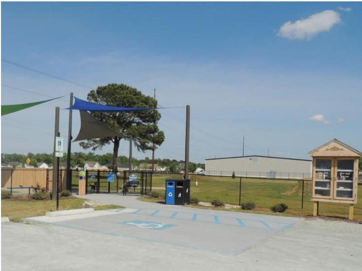
While the City of Dunn Dog Park has an ADA accessible space that is van accessible, the access aisle should be increased from a 5' width to an 8' width to be fully compliant.
