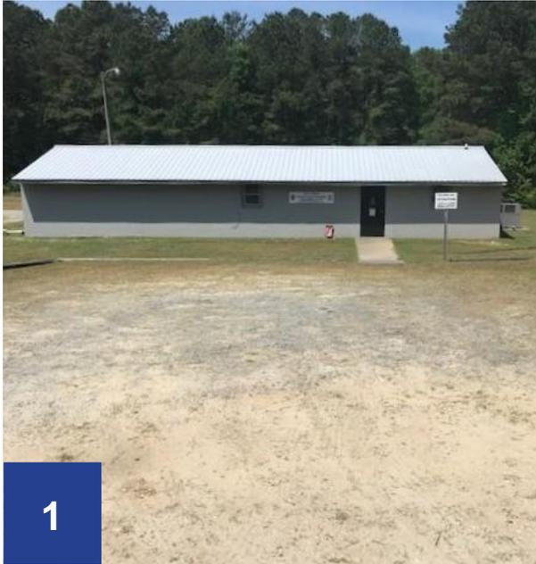
1. No accessible parking infrastructure exists. The parking area lacks signage, accessible spaces (including a van accessible space) and corresponding pavement markings, and an accessible route to the front entrance of the building.
