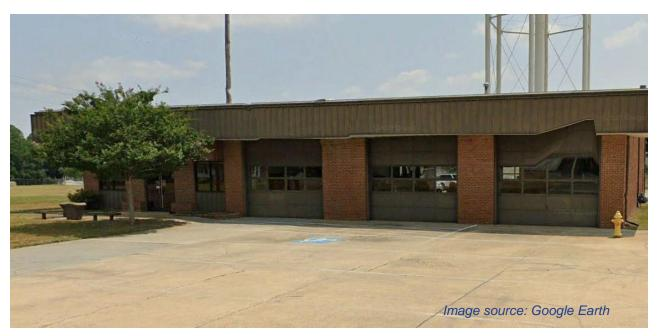
The parking area lacks adequate parking signage for the accessible parking space, which should also be designated as a van accessible space. An adjacent 8' access aisle is also missing next to the accessible parking space.
