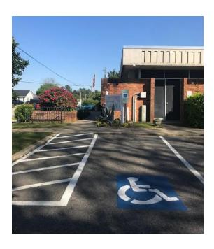
The library parking lot does not have a designated van accessible parking space. While an access aisle does exist, it does not meet the 8-foot wide minimum width for accessibility. Restriping the parking lot so that the existing accessible space and the space next to it become one van accessible space with an adjacent minimum 8' access aisle is recommended.
