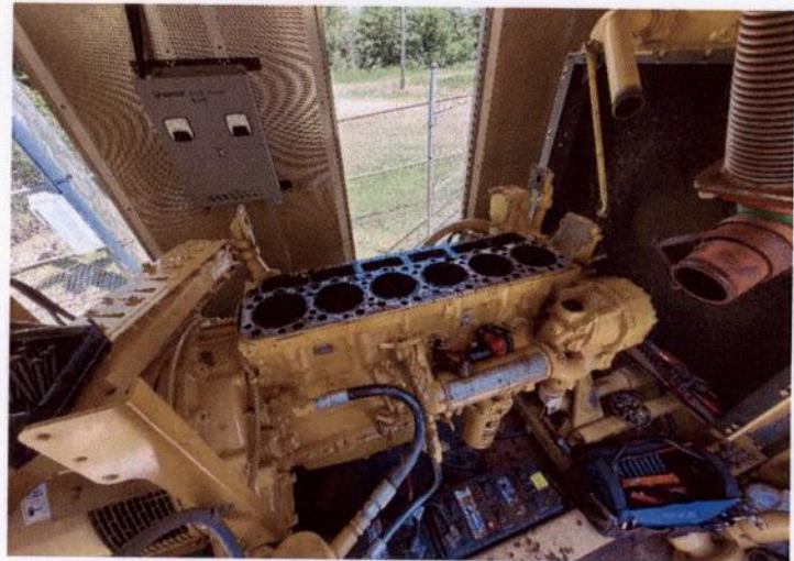
Side view of the engine. The head and gasket have been removed.
